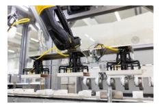
A six-axis robot erects cardboard inlays.
