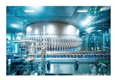
2) Filler and seamer part of the combined block solution SmartCan by KHS/Ferrum feature optimised hygienic properties.
